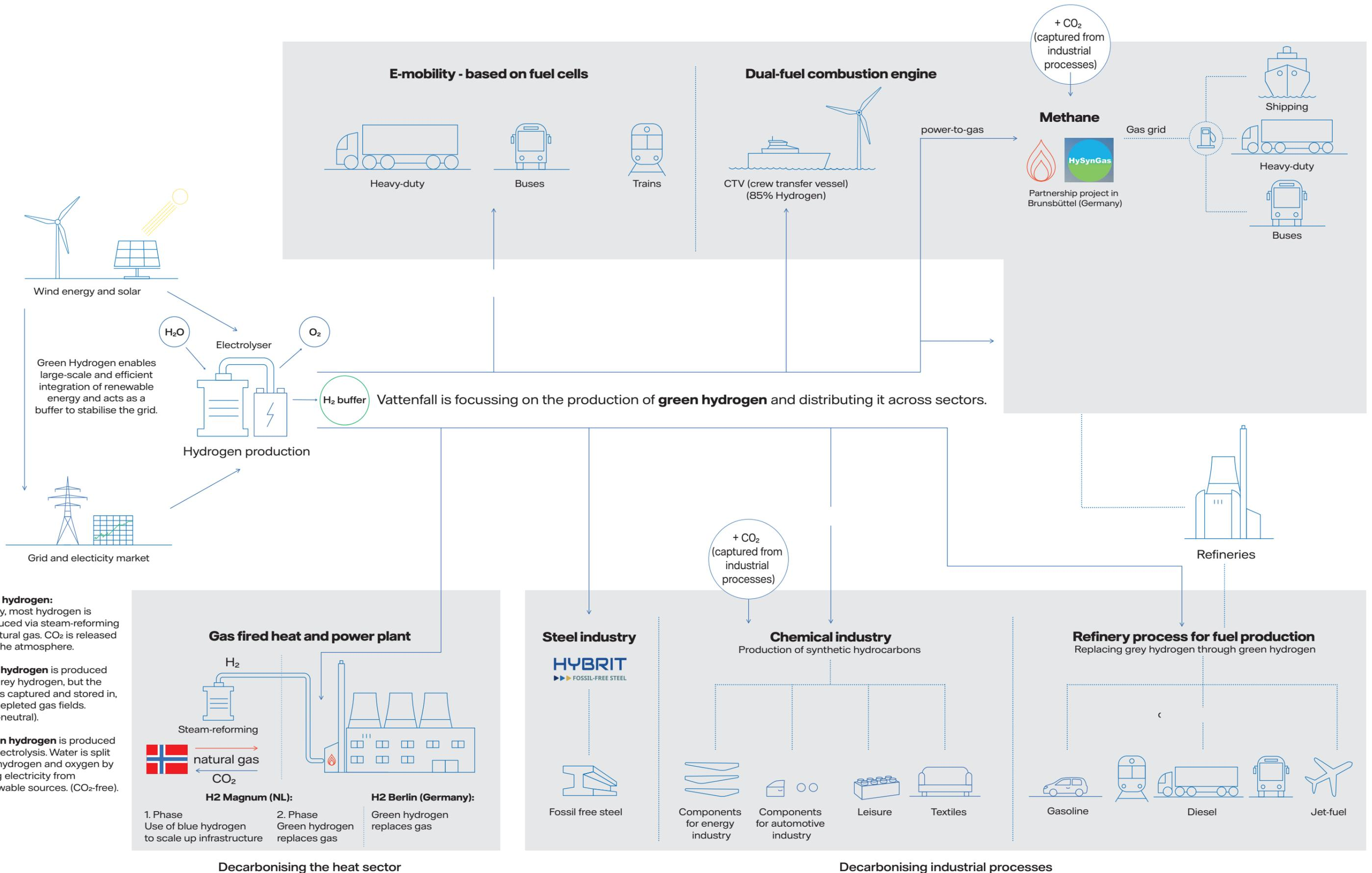
**Grey hydrogen:** Today, most hydrogen is produced via steam-reforming of natural gas. CO<sub>2</sub> is released into the atmosphere.
